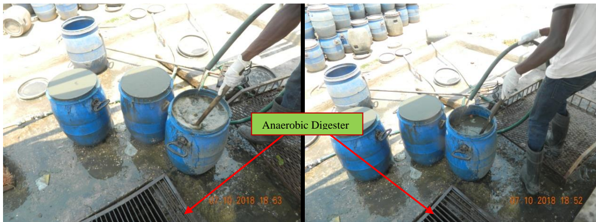
Figure 5. Washing of faecal sludge to separate the sludge from grit and solid waste, Kanyama study area.
