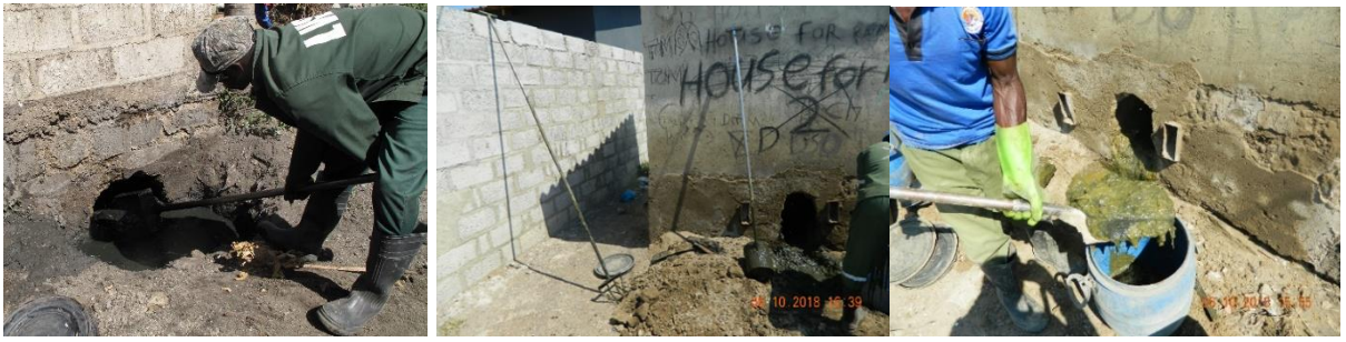
Figure 2. Sample collection: Left: A hole made on the side of the latrines; Middle: Some of the desludging tools including a modified garden rake and a 'Kanjote'; Right: Filling the barrel in the Kanyama study area.
